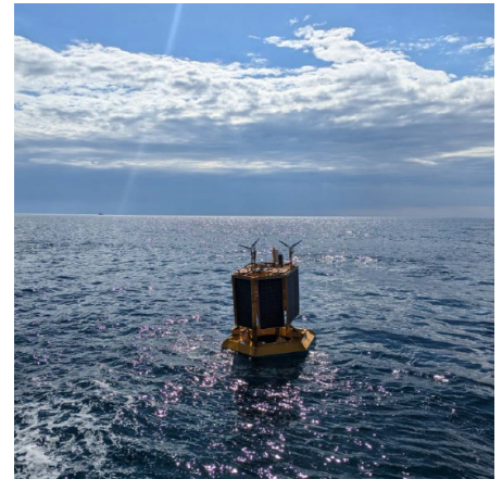
Floating LiDAR buoy
