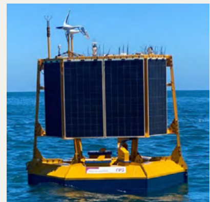
FLiDAR system – 4m x 4 m x 4m above sea level, keel 4.2m below the water line
